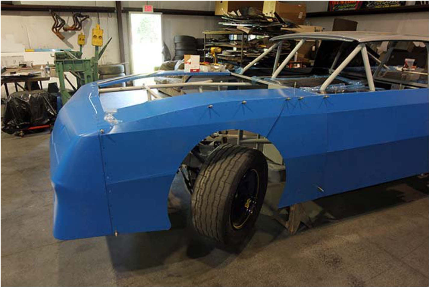
The finished fender, note the nice roll flare back to the cage.
