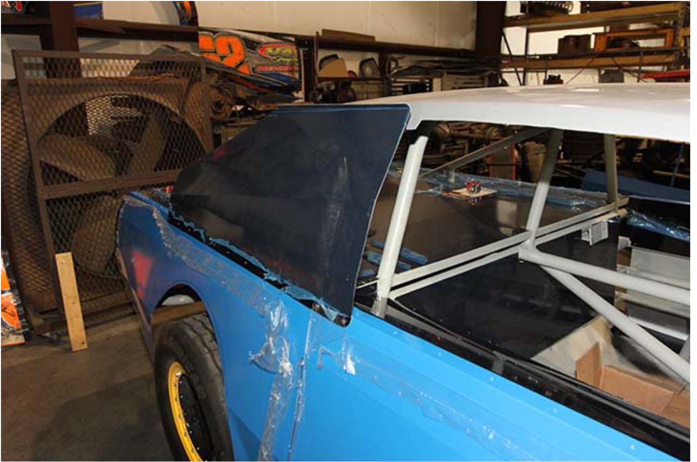
A large sail panel helps keep the rear of the car planted when it is thrown into the turns.
