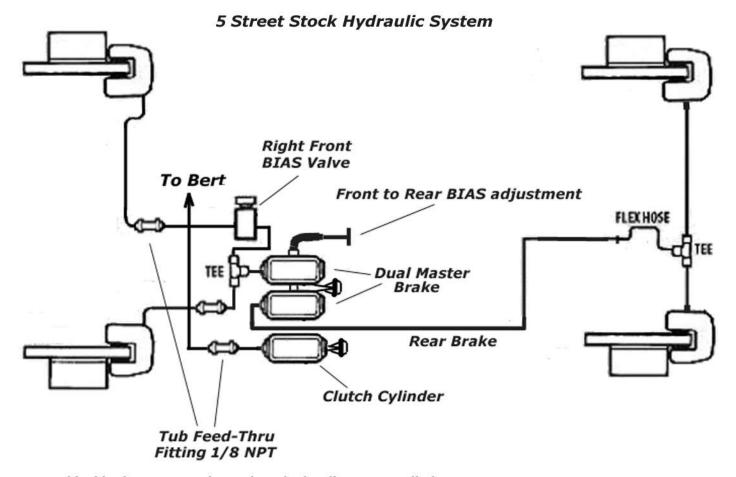
Located inside the racacer tub are three hydraulic master cylinders.
